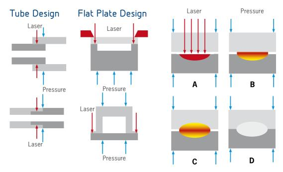
Laser light penetrates the upper layer and is absorbed by the lower material (A). The melting of the latter transfers (B) the heat to the upperlayer (C). The mutual melting pool solidifies under external pressure to a high-quality weld (D).
