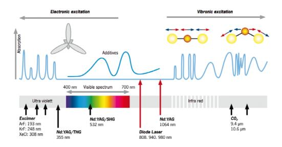
Most polymers (lighter blue curve) are usually transparent or transulent in the visible and near IR range. By adding pigments (darker blue curve), suitable absorption of the laser wavelength is achieved.
